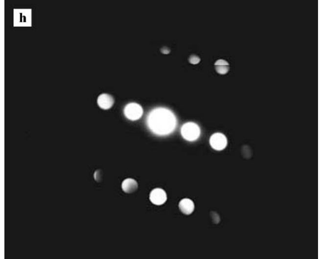
Fig. 2 cont. (e) diffraction patterns for rectangle plates; (f) fine V-rich carbides in clustering state, corresponding to diffraction patterns in (g) and (h)
